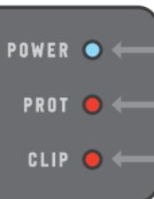
**POWER (blue LED):** Indicates amplifier operation when it is on.
