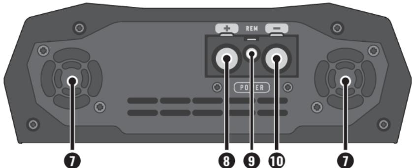
**7. COOLER:** Provides amplifier cooling. Install in a ventilated place, being careful to not obstruct the air vents.
