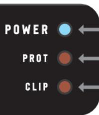
**POWER (blue LED):** Indicates that the amplifier is ON when it is lit up.
