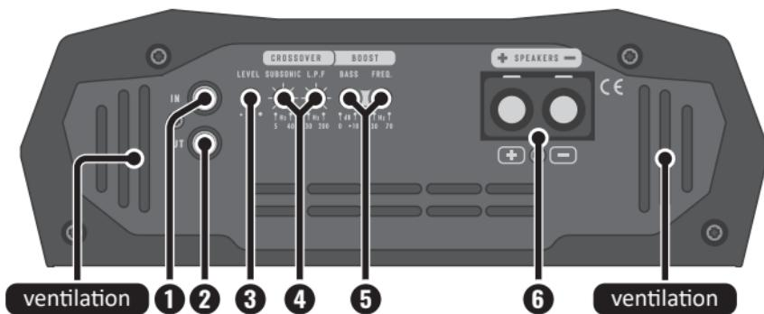
**1. INPUT (IN):** Input of the signal to be amplified. Connect to radio/player using high-quality RCA cables to prevent unwanted noise.
