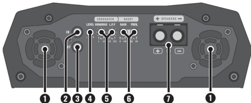
**1. COOLER:** Provides amplifier cooling. Install in a ventilated place, being careful to not obstruct the air vents.
