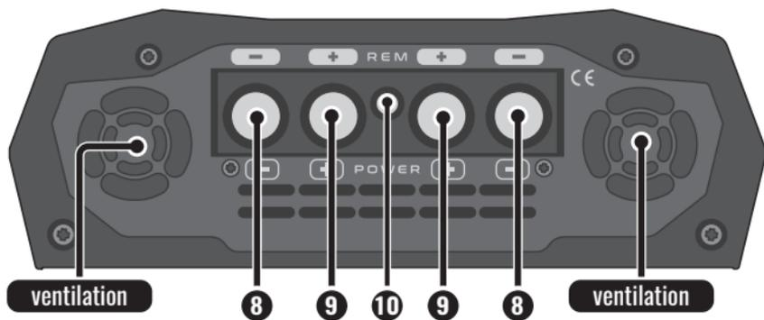
**8. DOUBLE CONNECTOR  $\ominus$  (GROUND):** Connect to the battery ground terminal using two cables of at least **00AWG** (one for each amplifier ground input).
