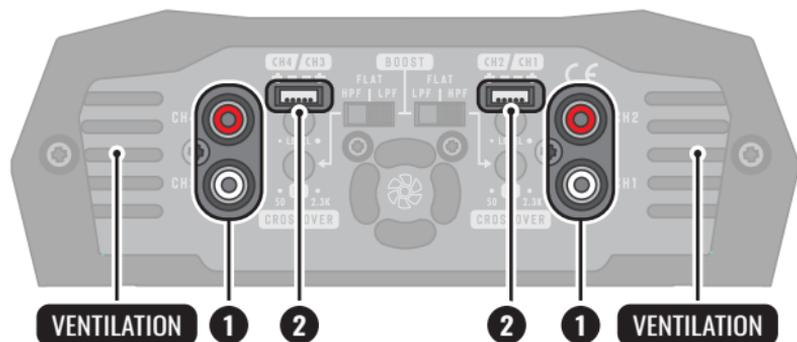
**1. RCA INPUT CONNECTIONS:** RCA double connections with 4 independent channels (CH1 and CH2 / CH3 and CH4) identified on the product. Connect to radio/player outputs via quality shielded RCA cables to prevent unwanted noise.
